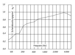
Sound absorption level – octave centre frequency (55 mm)
