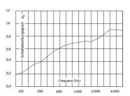
Sound absorption level – octave centre frequency (40 mm)
